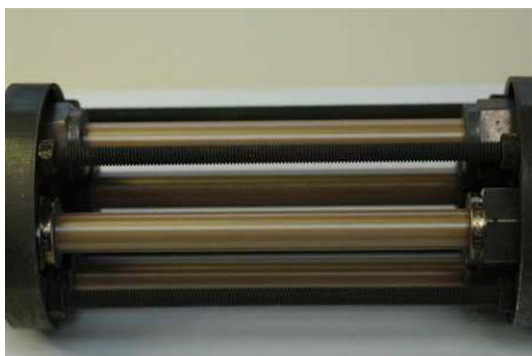
Fig. 1. Sample holder with four 12 cm-long oxidized claddings.
