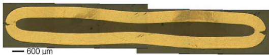
Fig. 4. Peanut-shape of a RXA Zy-4 ring after RCT at 20 °C. Optical micrograph on cross-section in the ring mid-section.
